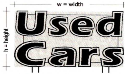
Calculating Area of a Sign where Copy Exceeds Sign Area = (height of copy) x (width of copy)
